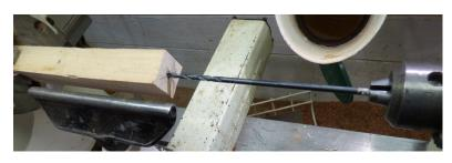
also drill from both ends but then you have to figure how to finish the end.
